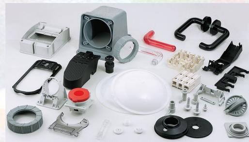
The cycle time of the plastic injection molding process can be broken down into the injection time, cooling time, and the resetting or changeover time. By reducing any of these times, production cost is lowered. Frequent mold changes allow inventory to be reduced and provide faster response to market requirements. The quick mold change systems from eas lower manufacturing cost by reducing changeover time.
