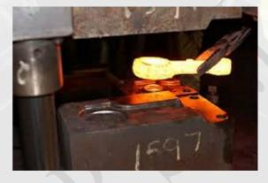
less material to remove. The close die forging process is typically used for critical components, in our case on railway, petrochemical, electrical, lifting and safety system, industrial and agricultural machinery sectors.
